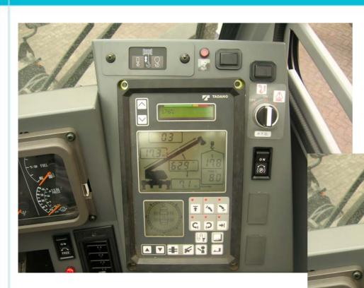
The crane operator had a history of overriding the crane limits and overloading the crane. Shown by computer records from the crane over 40 overloading incidents during October 2007
